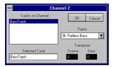
The **Channel Info** dialog box shows the MIDI tracks that are assigned to that channel and allows you to name them. There also is a **Transpose** function which lets you transpose the pitch of the selected track by octaves and/or semi-tones. Lastly, the **Patch** combo box provides an alternate way of selecting a patch for that channel.
